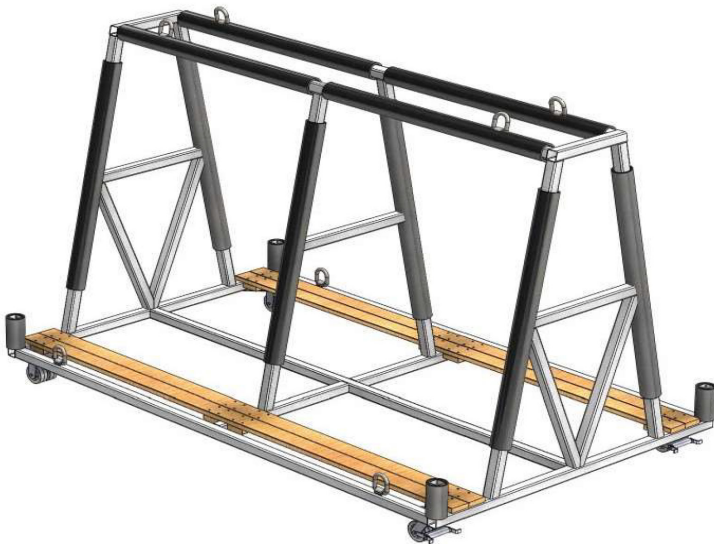
Left: Trolley used to transport the wings of the CF-100 designed by ÉTS students according to specifications drawn up by the QAM. Above: One of the two GPUs received from ÉNA. This provides either AC or DC power (ÉTS picture and Pierre Gillard photo).
