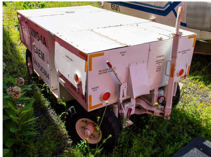
Left: Trolley used to transport the wings of the CF-100 designed by ÉTS students according to specifications drawn up by the QAM. Above: One of the two GPUs received from ÉNA. This provides either AC or DC power (ÉTS picture and Pierre Gillard photo).
