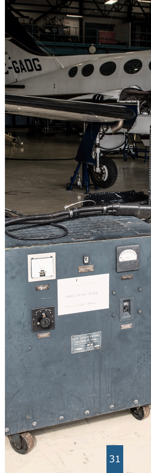
Left: Trolley used to transport the wings of the CF-100 designed by ÉTS students according to specifications drawn up by the QAM. Above: One of the two GPUs received from ÉNA. This provides either AC or DC power (ÉTS picture and Pierre Gillard photo).
