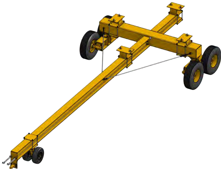
Above left: Trailer used to transport the fuselage of the Avro CF-100 Canuck designed by ÉTS students according to specifications drawn up by the QAM. Above right: One of the two GPUs received from ÉNA. This provides either AC or DC power (ÉTS picture and Pierre Gillard photo).
