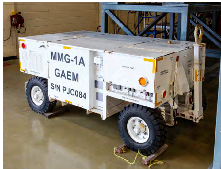
Above left: Trailer used to transport the fuselage of the Avro CF-100 Canuck designed by ÉTS students according to specifications drawn up by the QAM. Above right: One of the two GPUs received from ÉNA. This provides either AC or DC power (ÉTS picture and Pierre Gillard photo).
